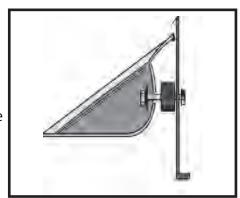
Step 7. Installing the front flares. First you will install the side marker in the flare using two phillips head screws. Install a 7mm rubber spacer on both marker light screws. Install one 7mm rubber spacer on the front mounting screw. Install a 13mm spacer on the remaining mounting screws. Mount the flare on the body placing a M5 nut on each bolt. Finally tighten the side marker screws. Do not over tighten the marker light screws or mounting nuts.
