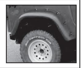
Step 9. Install the front flare extensions using the factory M5 bolts.
