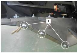
It's easier to install all the **45001113** before fitting the **46006973** and **46006974**.
